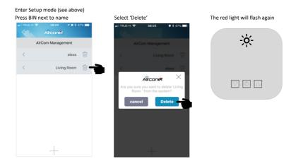
If the network red light on the thermostat does not flash after delete, need to reset the wifi from the thermostat itself by holding the  $\blacktriangledown \blacktriangle$  buttons for 10 seconds until all 3 Lights flash.
